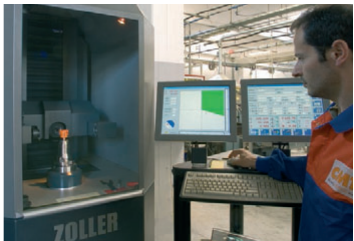
CMT's fully automatic measuring system.
