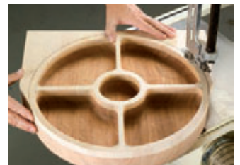
Bandsaw the exterior to final shape.
