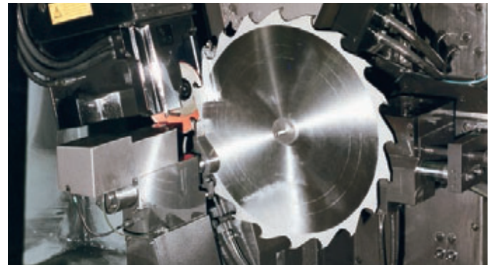
Sharpening the carbide tips.
