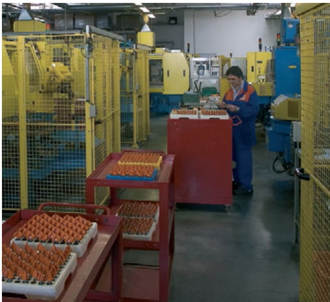
Loading the automated multi-axis CNC sharpening machines.
